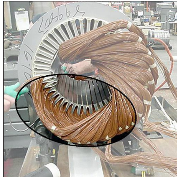
Figure 28. Lap winding showing all coils with the same span.
