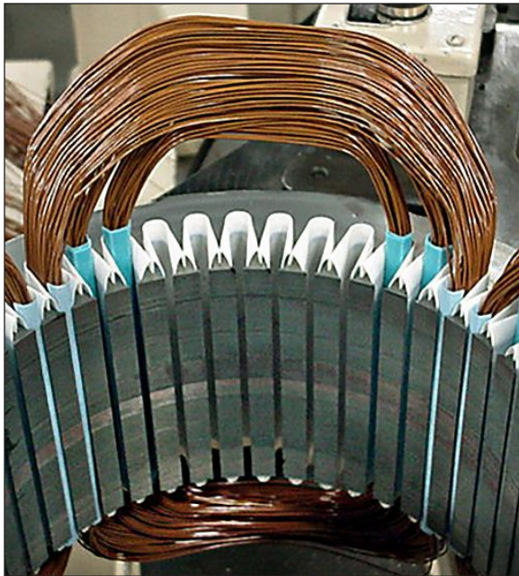
Figure 27. Typical concentric coil group. Note that each coil has a different span.
