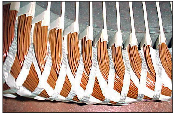
Figure 25. Typical coil extension for a 4-pole motor.
