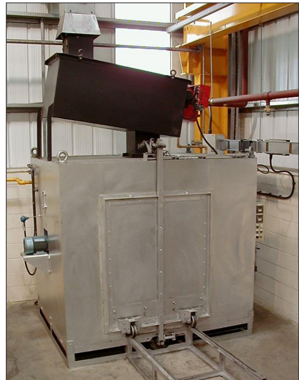
Figure 21. Controlled temperature burnout oven.
